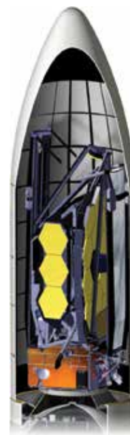
Drawing of the JWST folded into the Ariane 5 payload fairing. PHOTO CREDIT ESA
