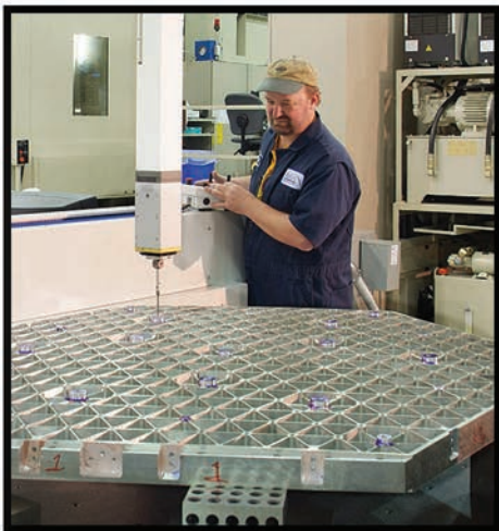
Axsys personnel use a Zeiss Prismo CMM on the shop floor to check parts at several points during and after processing.
