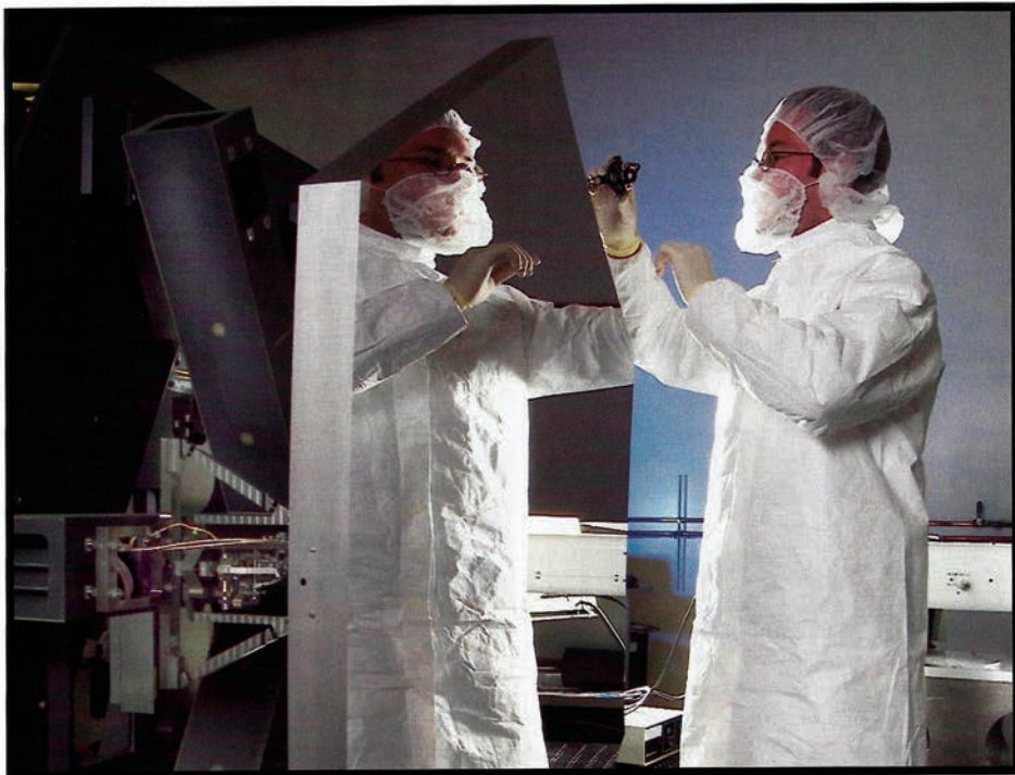
A technician mounts a fiducial (reference point) on the AMSD mirror segment, a technology demonstrator nearly as large as the JWST flight mirror segments.
