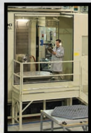
Eight modified Mitsui Seiki HS6A HMCs for the JWST mirror project are capable of volumetric positioning accuracy within a few microns over their 2000 x 1500 x 980-mm (X-Y-Z) machining envelope.
